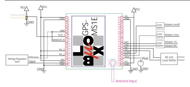
Figure 12: Recommended external wiring
